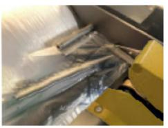
Thread the film through the pins and over the airpipe. Start production.
