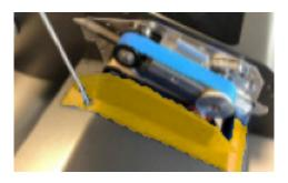
Fit the covers of the Teflon belts and screw it with the prepared hex key. Lower cover first and then the upper one.
