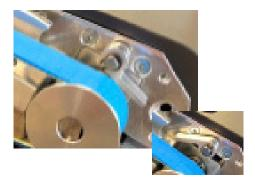
Turn the tension lever back to the left to press the transport rolls against each other.
