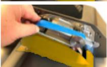
Now press the left roll to the right against the spring until it is possible to place the transport belt on the left roll.
