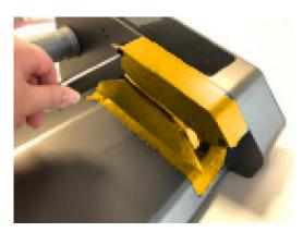
Undo both screws of upper cover with appropriate hex key and remove cover.
