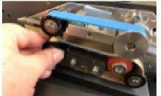
Push the lower of the two guiding rollers to the right against the spring to release the tension for the lower Teflon belt.
