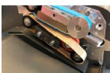
Remove the slackened Teflon belt from the rollers.
