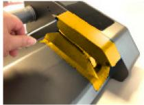
Undo both screws of upper cover with appropriate hex key and remove cover.
