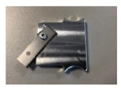
Fix the blade with the corresponding screw.
